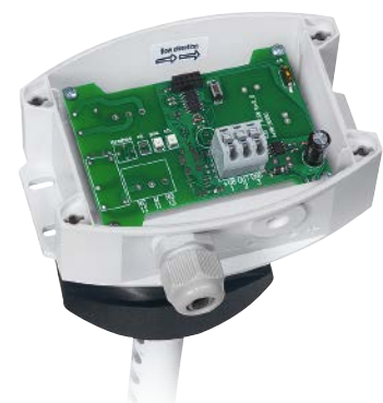
KLGF-U with output 0-10V, UB = 24 V
