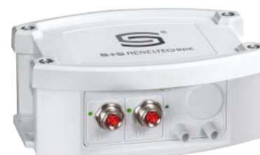
EtherCATP Cable connection and LED status display
